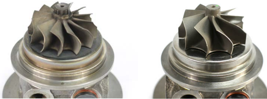
Figure 11: Standard 12-blade turbine wheel (left) and high flow 9-blade turbine (right).
