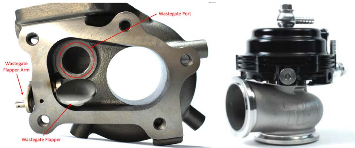
Figure 8: Typical internal wastegate design (left) and typical external wastegate design (right).
